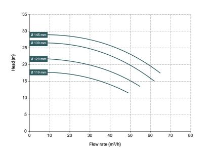
The curves and the performances refer to pumps with immersed suction and open delivery outlet, with water at 20°C and vary based on the composition materials and 50 Hz two-pole motor (2900 rpm).
